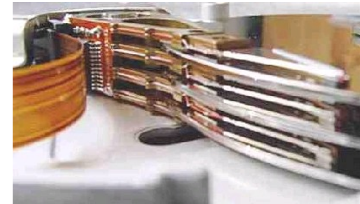
Read/Write Head Side View
